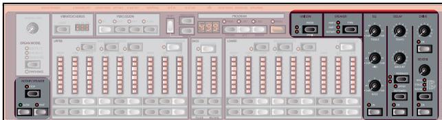
The Effect Section is where you set and adjust settings for delay, drive, EQ, unison, reverb and speaker simulation. Please refer to “The Effect Section” on page 13.
