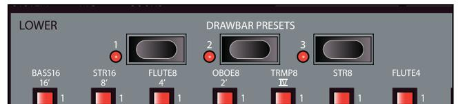
The **PRESET** buttons lets you change back and forth between different drawbar set-ups instantly. Changes are automatically saved and recalled the next time you activate the same preset.
