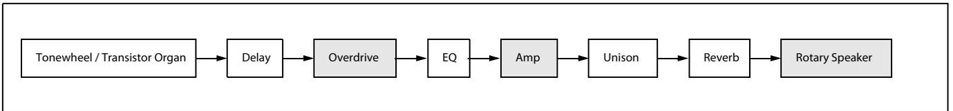
The *Overdrive*, *Amp* and *Rotary Speaker* models are used one at a time, depending on the **SPEAKER** button setting.
