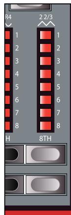
The drawbars of Nord C1 Combo Organ behave similar to their mechanical counterparts, i.e. with the Tonewheel and Electric-V models you "pull out" and "push in" the drawbars using the **DRAWBAR** buttons. The buttons are special in the way that they auto-increment/decrement the drawbar value when held. I.e. if you hold a **DRAWBAR** button the corresponding drawbar value will continue to increment or decrement (within its range) until you release the button.
