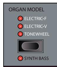
You select which model to play using the **ORGAN MODEL** button. Only one model can be used at a time.
