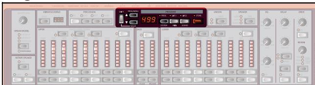
The Program Section is where you store and recall sound settings into Programs, and also adjust system specific parameters. Please refer to “The Program Section” on page 8.
