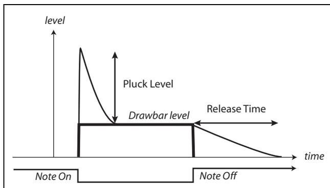
Pluck and release time are adjusted with the **BASS** drawbars while holding down the **SHIFT** key.
