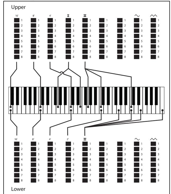
The two rightmost drawbars control the sum of all partials in the form of a filtered triangle-like signal sounding soft and dark, and an un-filtered square signal sounding bright and intense.
