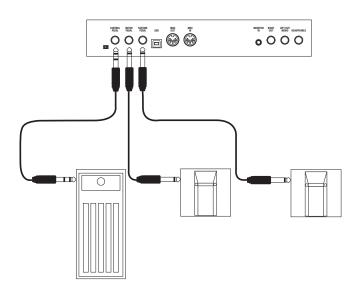
The Nord Electro 4D has three pedal inputs; a sustain pedal, a pedal to control the rotor speed and a control pedal (an expression type pedal), which can be used to control various parameters.
