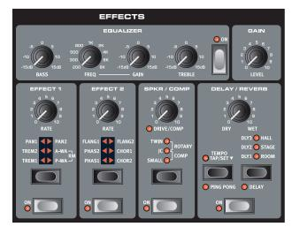
The Effects section of Nord Electro 4D can be used for processing the organ and piano/sample sounds. It is programmable and you can configure your effects separately for each program.
