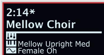
A Program contains all the settings for all of the available parameters, including sound engines and sound processing effects, for both Parts regardless of whether both Parts are active within the Program. Output volume of each Program is controlled using the **GAIN** knob. This value is also stored within the Program, allowing adjustment of relative volumes between Programs.
