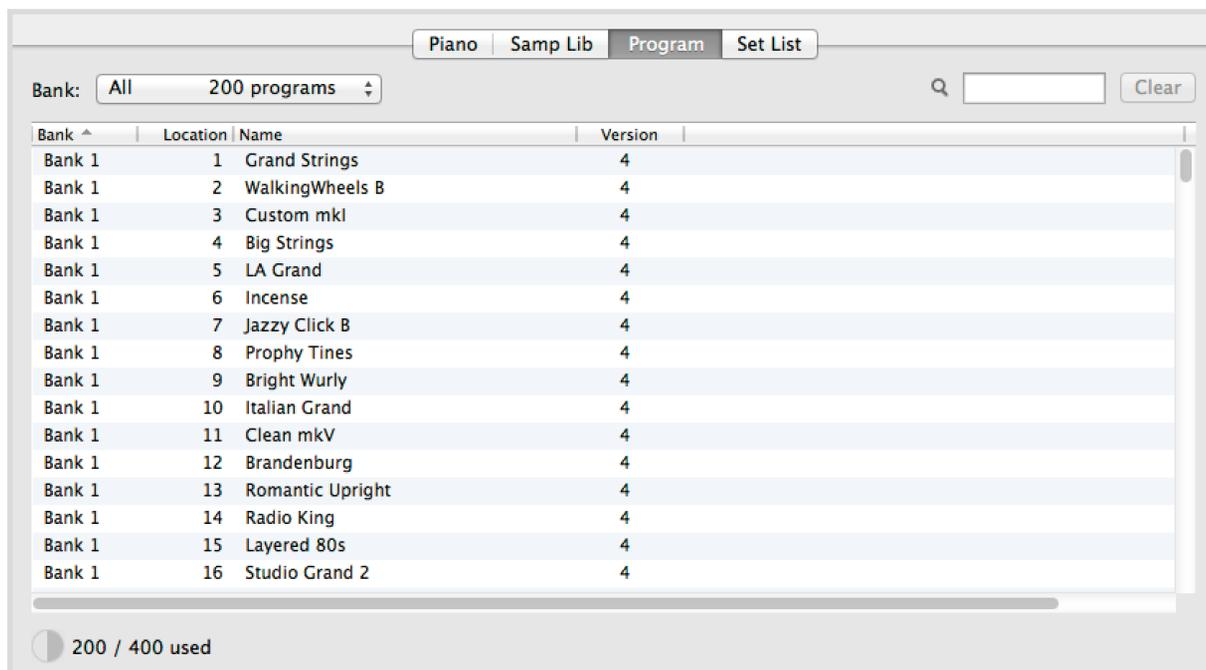
The main area of the Nord Sound Manager is the list view, divided into tabs representing the four partitions: **Piano**, **Samp Lib**, **Program** and **Set List**. Within each tab the content of the partition is listed. At the top of the list view is a dropdown Bank selector and at the bottom a Partition Memory Indicator, showing how much of the space within each partition is being used.
