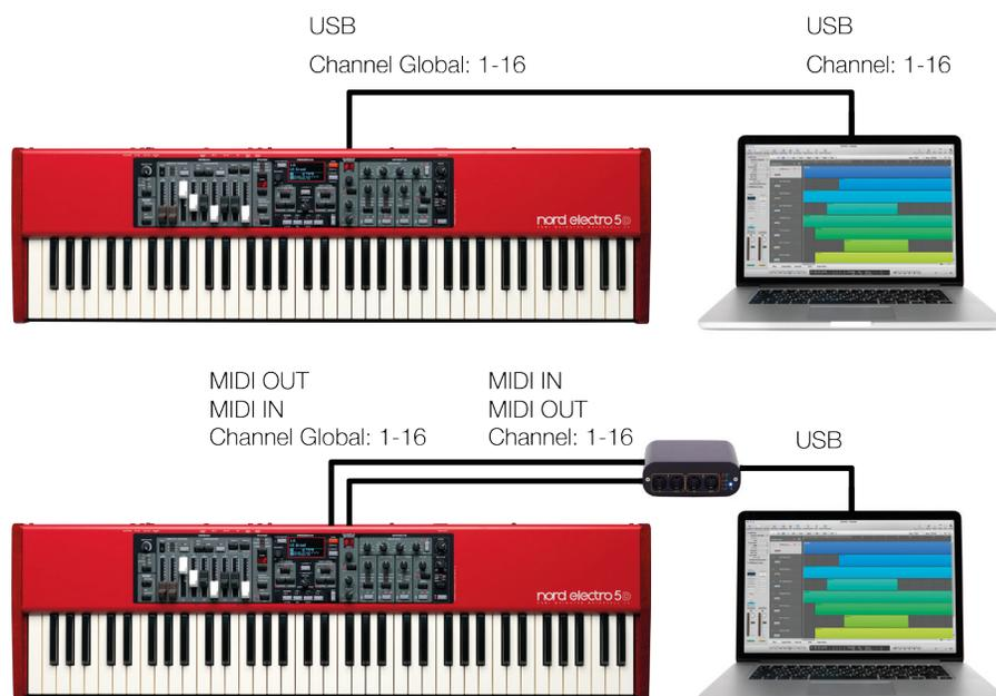
**MIDI Connections:** Connect a USB cable between the Nord Electro 5 and your computer, or a 5-pin MIDI cable between the MIDI OUT of the Nord Electro 5 and the MIDI IN of your MIDI interface.
