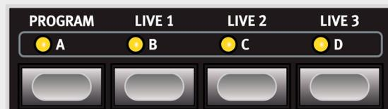
The Nord Electro 5 has three easy-to-access Live Programs, differing from regular Programs in that edits you make are automatically stored. Even when exiting a Live Program, or powering off the machine your sounds will remain the way you left them, without the need for storing.
