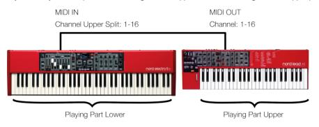
MIDI Connections: Connect a 5-pin MIDI cable between the MIDI IN of the Nord Electro 5 and the MIDI OUT of the external keyboard.
