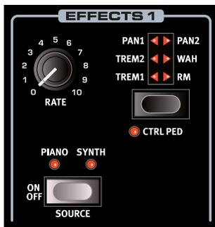
The **EFFECTS 1** unit offers six different types of modulation effects. Use its Selector button to switch between the available settings, and the **RATE** knob to set the rate (speed) of the selected effect.
