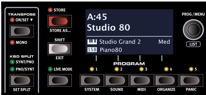
The centrally located Program section provides access to performance functions such as loading and storing programs, access to Live programs, keyboard split functionality and more. This is also where menus containing *System*, *Sound* and *MIDI* settings are found. The menus and their settings are covered in a separate chapter, starting on page 22.
