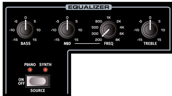
The three band equalizer features bass, sweepable midrange and treble controls.
