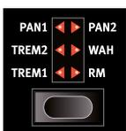
*Selector* buttons are used to select one setting in an array. They have a set of round or triangular LEDs to indicate its current setting. Press the button several times to cycle through the possible options.
