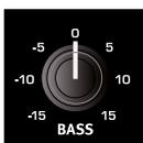
Potentiometer-type *knobs* are used for many parameters on the Nord Grand. When a program is loaded the physical positions of these knobs will in most cases not correspond to the actual parameter values. As soon as a knob is turned however, its associated parameter value will “snap” to the knob's position.
