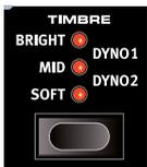
Use the Piano **TIMBRE** settings to quickly alter the character of the selected piano sound – while keeping the EQ unit of the Effects section free for other tasks.
