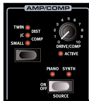
The **AMP/COMP** unit includes sophisticated amplifier and speaker cabinet simulations, a versatile tube distortion setting and a useful compressor effect. The amount of drive or compression is controlled with the **DRIVE/COMP** knob. The LED indicates whether any overdrive is active, and will light up whenever the compressor is working.
