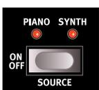
**ON/OFF** buttons are used for activating a function or a group of functions such as effects and have a LED close to them to indicate the on/off status and sometimes also the source or zone.
