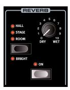
The **REVERB** unit simulates the natural sound reflections in various acoustic environments. The Reverb is a "global" effect, which is to say that it is always applied to *all* active sound engines.
