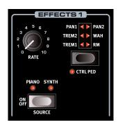
The **EFFECTS 1** unit offers six different types of modulation effects. Use its Selector button to switch between the available settings, and the **RATE** knob to set the rate (speed) of the selected effect.
