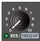
The Resonance (**RES**) parameter is used to further adjust the characteristics of the filter. Increasing the Resonance will emphasize frequencies around the cutoff frequency, making the sound thinner.
