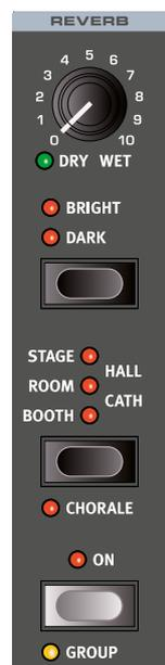
The **REVERB** unit simulates the natural sound reflections in various acoustic environments. There are five reverb types of various lengths and densities, indicated by the LEDs in the selector.
