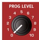
The **PROGRAM LEVEL** knob determines the overall sound level of a program, and is stored with the program unlike the Master Level control. Use this control to maintain equal levels between programs, without needing to adjust all 4 layer faders.
