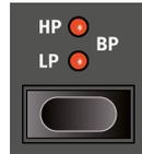
*Selector* buttons are used to select one setting in an array. They have a set of round or triangular LEDs to indicate its current setting. Press the button several times to cycle through the possible options.
