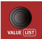
The *dials* on the Nord Wave 2 are knobs without any fixed start and stop positions, used for navigating parameters and settings in a step-wise fashion. The **VALUE** dial is one such example. In this manual, dials are sometimes also referred to as *encoders*.
