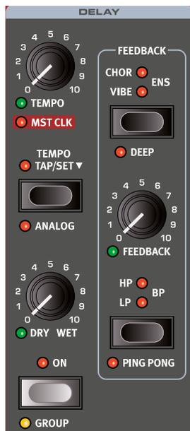
The **DELAY** unit produces echo/repeat effects. The Delay time is set with the **TEMPO** knob, or can be tapped using the **TAP** button.
