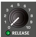
Knobs that can serve as a Morph destination are equipped with green Morph LEDs. These are located at the bottom left of the knob, and will light up if a Morph is targeting that parameter. Read more about Morphs on page 16.
