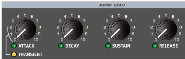
The Amplifier Envelope (**AMP ENV**) is used for controlling how the sound *level* changes over time. By modulating the amplifier with an envelope, the sound can be given its basic profile and evolving character. In fact, the “volume shape” is one of the most important factors to how we identify the sound. By setting up a proper amplifier envelope you can make a sound “soft”, “hard”, “plucked” “static” etc.
