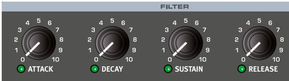
The Filter Envelope, with controls for **ATTACK**, **SUSTAIN**, **DECAY** and **RELEASE** works on the same principles as the Amplifier Envelope – see above – except that it is used for modulating the filter cut-off frequency rather than the amplifier level. The amount of modulation is determined by the Env Amt control.
