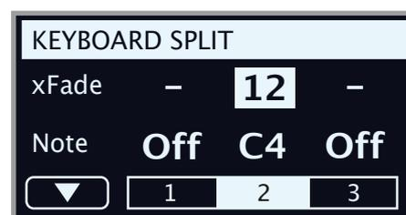
Select the split point to adjust by pressing its soft button (1, 2 or 3) and turn the dial to change its setting.
