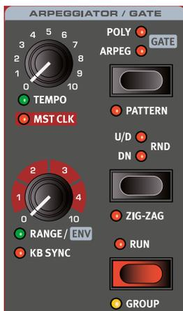
The Arpeggiator/Gate section is turned on by pressing its **RUN** button. Activating **GROUP** (Shift + Run) allows multiple layers to share the same settings. Read more about Group on page 23.
