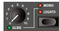
In both **MONO** and **LEGATO** mode only one note is played at a time, just like on a traditional monophonic synthesizer. The main difference between the two modes is in how the modulation and amplifier envelopes act when one is *playing* legato, i.e. with overlapping key presses:
