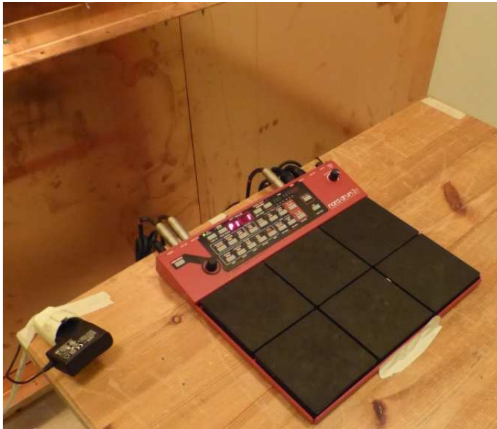
Photo of the test set-up for conducted emission
