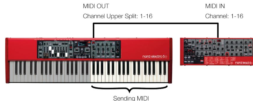
*MIDI Connections:* Connect a 5-pin MIDI cable between the MIDI OUT of the Nord Electro 5 and the MIDI IN of the external module.
