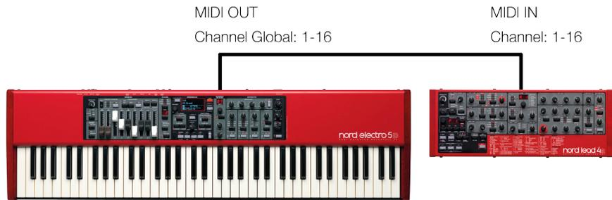
*MIDI Connections:* Connect a 5-pin MIDI cable between the MIDI OUT of the Nord Electro 5 and the MIDI IN of the external module.
