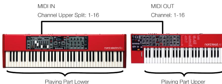
**MIDI Connections:** Connect a 5-pin MIDI cable between the MIDI IN of the Nord Electro 5 and the MIDI OUT of the external keyboard.
