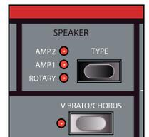
When using an external cabinet connected via the high level outputs the **ROTARY SPEAKER**'s LED will flash repeatedly if activated to indicate that the internal rotary speaker simulation is bypassed. Please note that this is dependant on the external cabinet circuitry, and if the LED do not flash but lit constantly you will experience a double rotary speaker effect.
