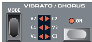
**B3** – The original tonewheel organ's vibrato and chorus scanner consists of a tapped delay line in combination with a rotating scanner. For the Vibrato effect, phase shift is applied to the signal. For the Chorus effect, a phase modulated signal is added to the original signal. Three different types of choruses (C1- C3) and three different types of vibratos (V1-V3) are available.
