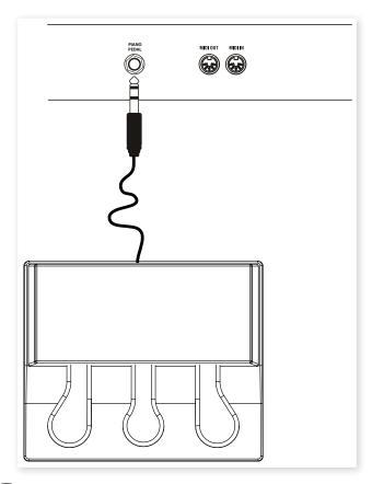
(1) Connect the ¼" stereo connector from the Nord Triple Pedal to the Piano Pedal connector on the Nord Piano.
