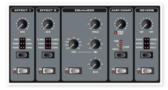
The Effects section of Nord Piano can be used for processing the piano sounds. It is programmable and you can configure your effects separately for each and every program. Some of the effects are mono in/ Mono out and some are stereo in/stereo out. For each individual effect the channel configuration is stated in the related text.
