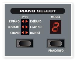
The Piano section of the Nord Piano is organized into six types; each type can contain several instrument models. You can freely add new piano instruments via USB using the Nord Sound Manager utility (read about the Manager on page 18).
