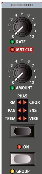
The **EFFECTS** unit offers six different types of modulation effects. Use its Selector button to switch between the available settings.
