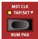
The Master Clock allows you to synchronize the Arpeggiator/Gate, the LFO, the Delay and Effects Rate in the Nord Wave 2. Not only can these be made to run in sync with each other; different subdivisions can be set for all synced components, allowing for some great rhythmic effects.
