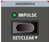
The **IMPULSE MORPH** feature allows for instantly changing one or more parameters at the press of a button, for dramatic or subtle changes in sound. Apart from all parameters that are available as morph destinations for the continuous morphs described above, the Impulse Morph can change various button controlled parameters, such as Filter Type, or turning the Arpeggiator/Gate on or off.
