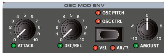
The **PITCH** (Semitones) or **OSC CTRL** parameter for the Oscillator (read more about this below) can be modulated by the dedicated Oscillator Modulation Envelope.
