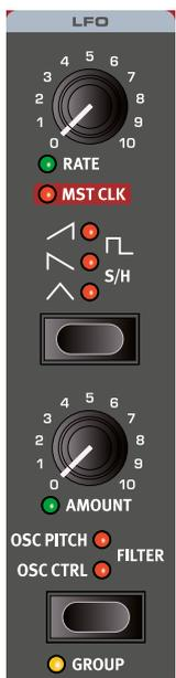
The Low Frequency Oscillator (**LFO**) produces a waveform that can be used to create cyclic modulations to the selected destination; Oscillator Pitch (**OSC PITCH**), Oscillator Control (**OSC CTRL**) or the Filter cut-off frequency (**FILTER**).
