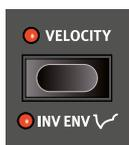
When **VELOCITY** is turned on, the modulation amount for the Filter Envelope is controlled by how hard the key is being played.
