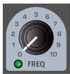
The filter **FREQ** knob is used for setting the *cut-off frequency* point – that is where in the frequency range the filter begins to process frequencies. The actual result of this processing depends on the type of filter used.
